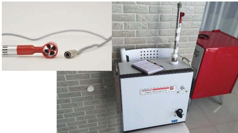
Figure 2. Meteorological sensor used on monitoring the balconies
