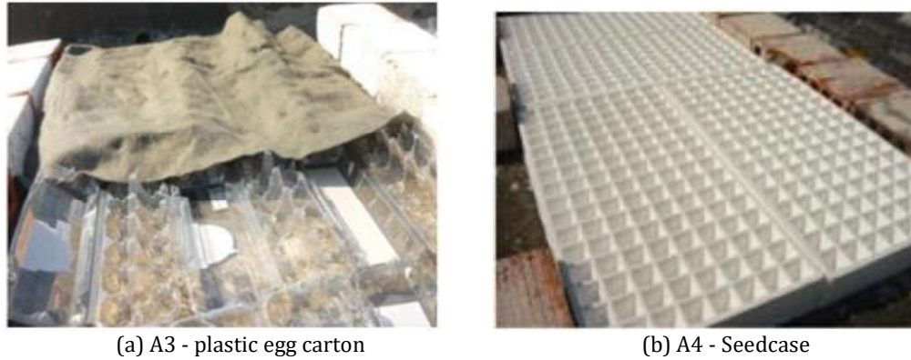
Figure 3a-b. Experiment 1 - Devices made for rainwater storage (a) A3; (b) A4
