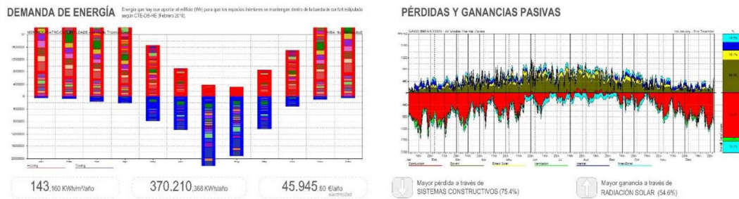
Figure 3. CASE 0 – Current status. Monthly demand for energy. Passive lost and gains. (results by ECOTECH)
