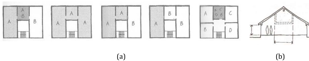
Figure 4: (a) neutral environments for different uses; (b) Usable Attic: adequate ceiling height and structural system. Source: (a) Schneider & Till (2007, p. 189); (b) Hamdi (1991, p. 99).
