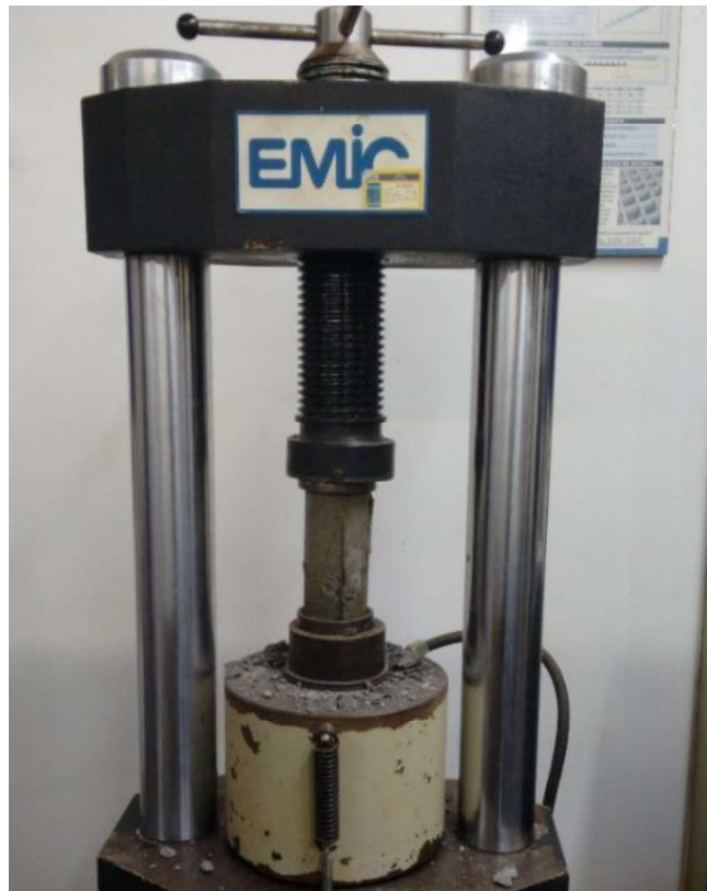
Figure 1. Axial compression strength test. Source: Authors, 2016
