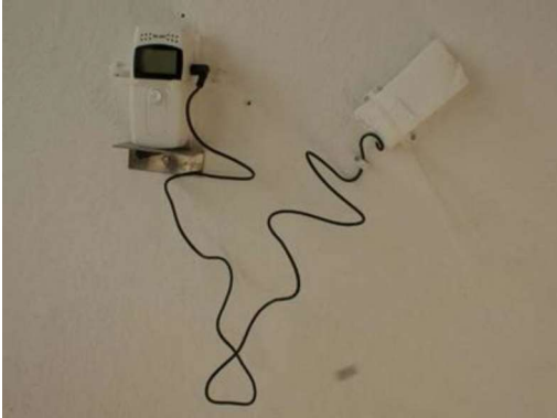
Figure 14. View of data logger to measure surface surface temperatures
